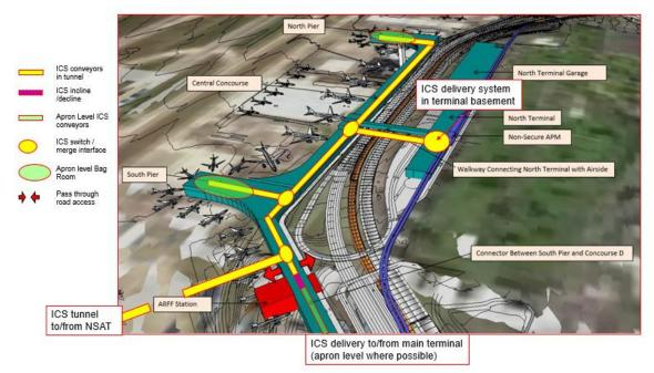
Figure 3 View illustrating ICS connectivity at North Terminal
