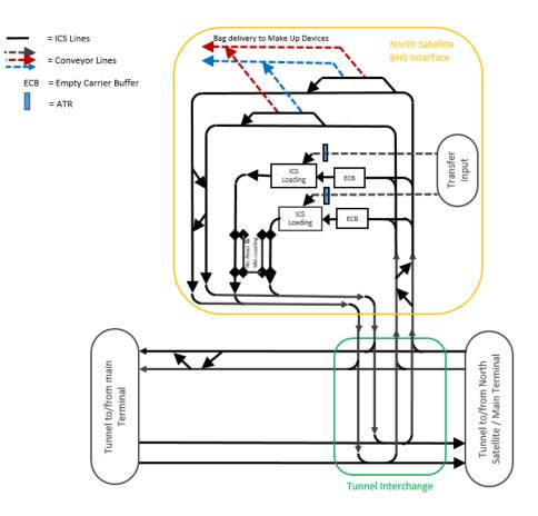
Figure 25 ICS connectivity North Terminal to North Satellite bag room
