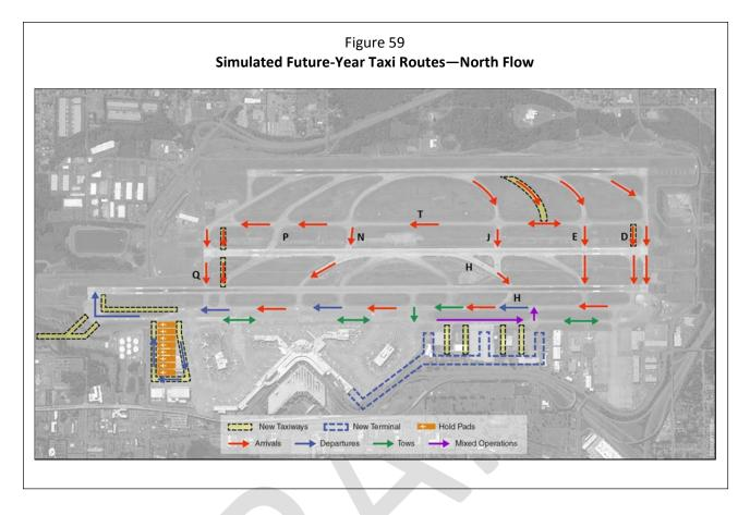
Four crossing points were simulated in South flow, and seven crossing points were simulated in North flow. South flow supported fewer crossing points than North flow due to the location of the departure queue.
