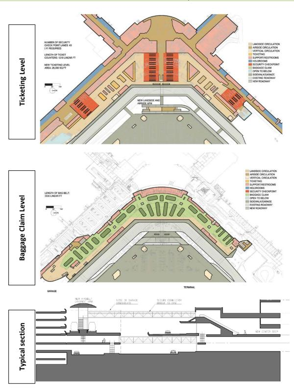
Figure 3-10 Concept 4 – Expand Center of Terminal to East, Provide Secure & Non-secure APM Seattle-Tacoma International Airport
