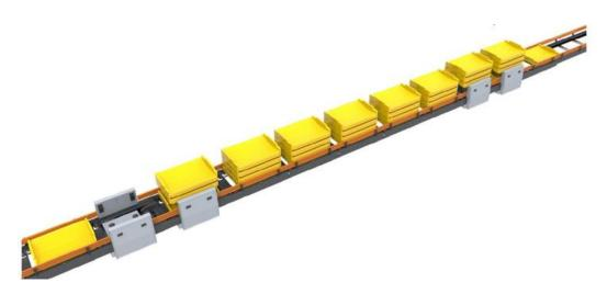
Figure 15 In-line empty carrier storage ECB (source Vanderlande)
