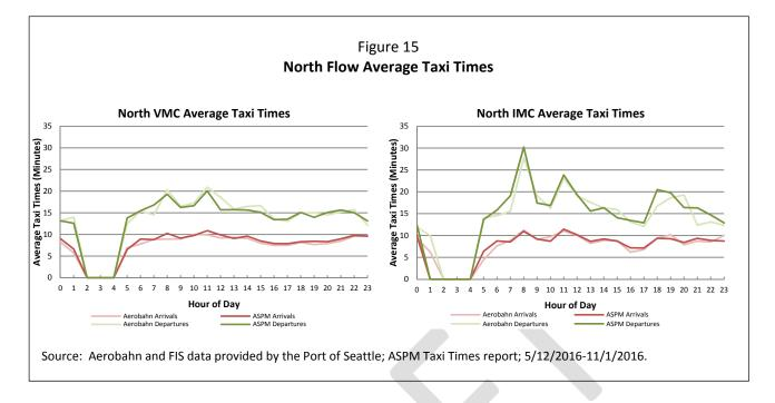
The results show that ASPM and Aerobahn/FIS taxi times tend to agree, which suggests that Aerobahn/FIS data may be used to estimate taxi times.
