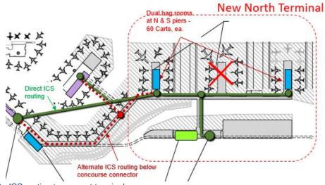
Figure 2 Alternate ICS routing to connect terminal areas
