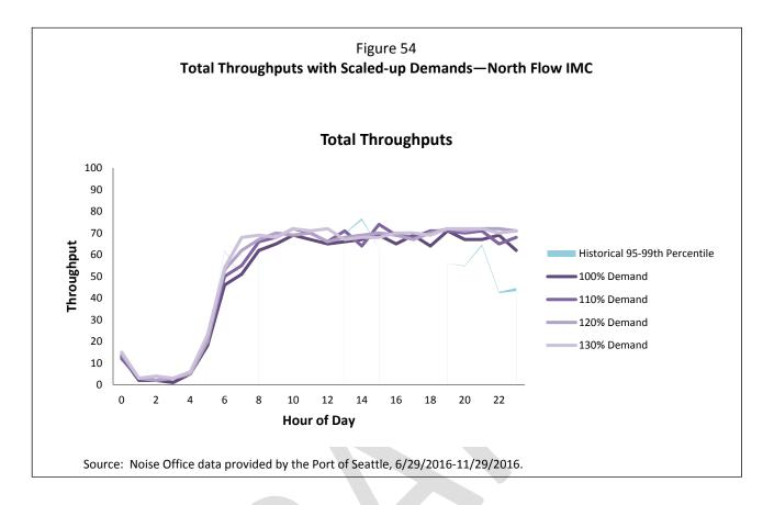
All five of the models achieved saturation at 130% of the current demand level. Many of the maximum achieved throughputs fall between the 95<sup>th</sup> and 99<sup>th</sup> percentile of observed hourly throughputs, suggesting that the airfield occasionally reaches its capacity measured on an hourly basis.
