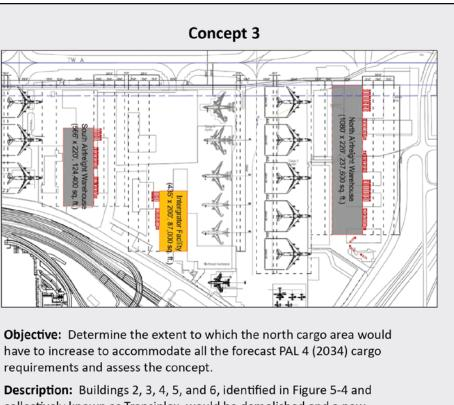
Assessment: A new 237,600 square feet multi-user air freight warehouse and five air freight hardstands would be located on the Transiplex site. The warehouse would be deficient by 124,400 square feet at PAL 4 (2034). An 87,000 square foot integrator warehouse would be located on the FedEx site. A 124,400 square feet warehouse and three air freight hardstands would be located to the south of FedEx. The hardstands deficient by three positions (two of
