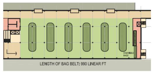
Figure 1 Proposed domestic claim layout, North Terminal
