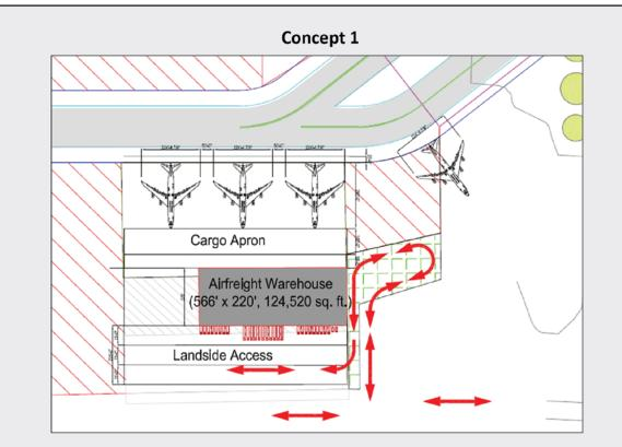
**Objective:** Provide airfreight warehouse capacity and freighter parking positions to supplement the facilities provided in the north cargo area.
