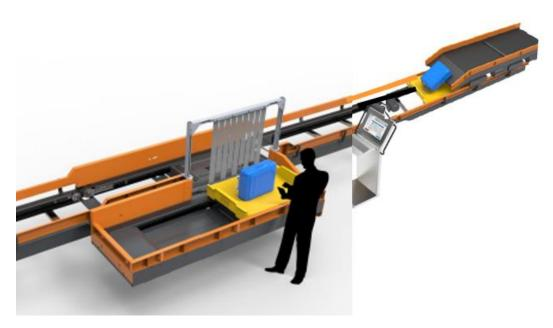
Figure 9 Bag induction and manual encode/mis-load station
