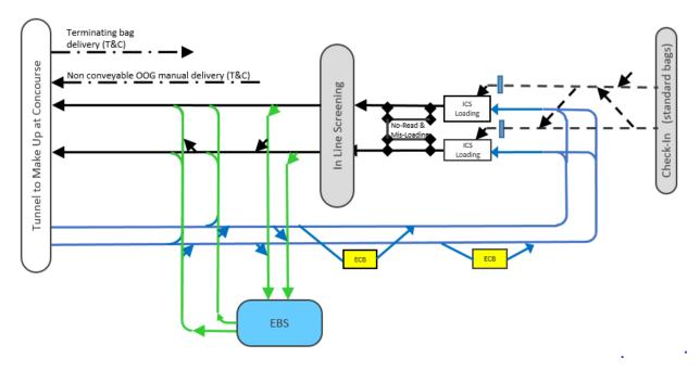
Figure 16 Modified MFD providing ECB storage in tunnel
