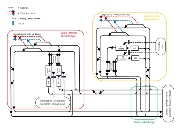
Figure 22 Overview of ICS delivery/sortation connectivity, North Terminal to other terminal areas
