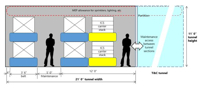
Figure 17 Modified tunnel configuration with ECB storage in tunnel
