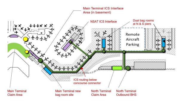
Figure 21 Possible Inter-Terminal connectivity of BHS facilities by ICS delivery/sortation system
