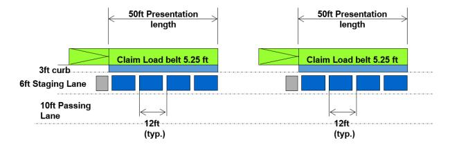
Figure 6 Possible layout approach for claim load belts
